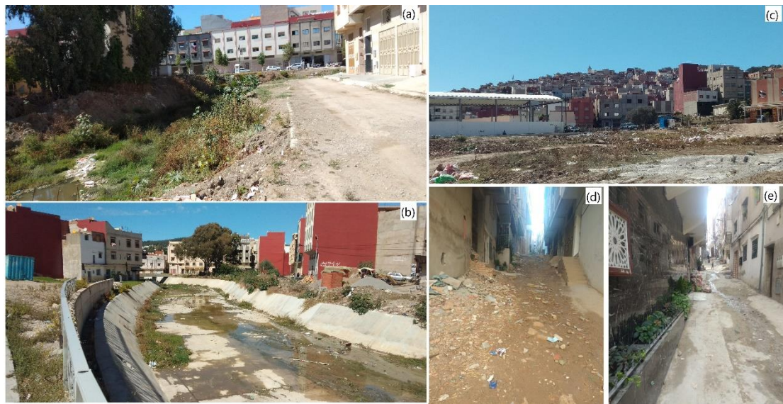
Figure 9. Example of areas in Tangier city identified by all four models as being at very-high vulnerability of flooding: (a,b) associated with short distance to the channel, high drainage density and recent buildings; (c–e) associated with steep slopes, high density of old buildings and high population density.
