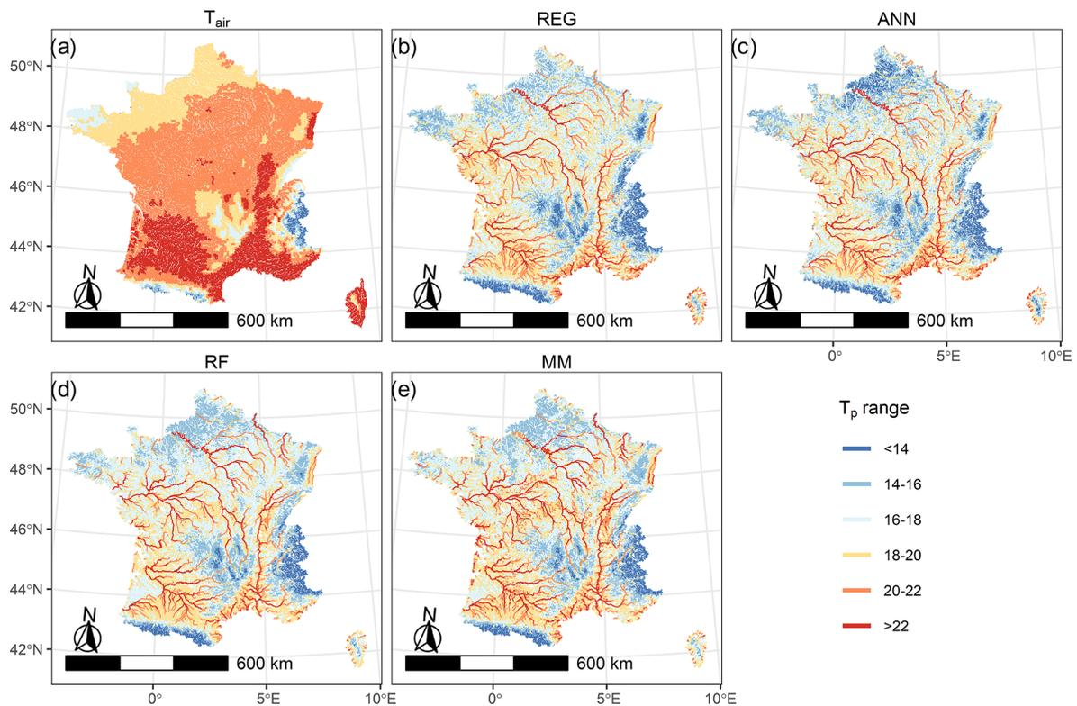
**Figure 6.** Thermal peaks ( $T_p$ ) of stream water extrapolated to all reaches of the French hydrographical network RHT with the different predictive model structures: (a) air temperature ( $T_{air}$ ), (b) multiple regression (REG), (c) artificial neural network (ANN), (d) random forest (RF), and (e) multi-model combination of all previous models (MM). All reaches are colored by their modeled range of  $T_p$ , and colors are chosen to improve visualization.
