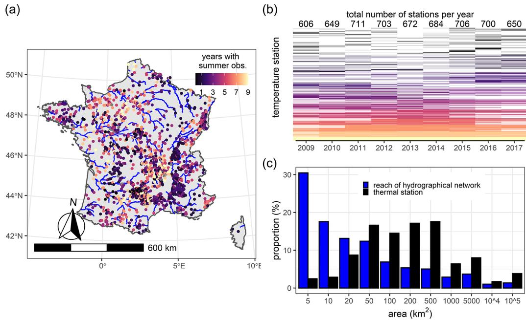
**Figure 1.** Data availability for each temperature station used in this study. **(a)** Map of stream temperature stations in France with RHT network shown for all reaches of Strahler order  $> 4$ . **(b)** Heatmap of data availability by year (x axis) and station (y axis) with the total stations per year listed at the top of each column. Sites are colored by the number of years with observations. **(c)** Distributions of drainage area for RHT reaches (blue) and of thermal stations (black).
