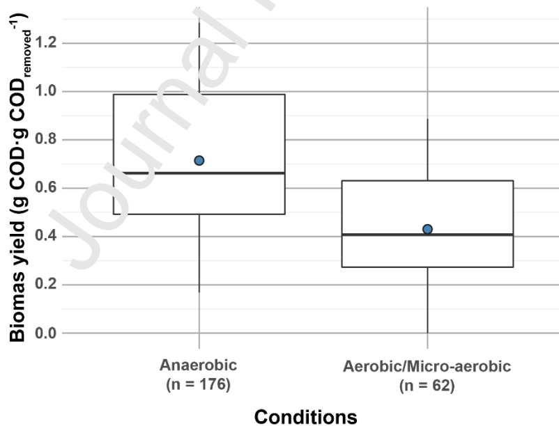
Figure C1. Biomass yields under anaerobic and aerobic/micro-aerobic conditions (dissolved oxygen between 0.5-8.0 mg·L -1 ). The blue dots represent mean values. COD stands for chemical oxygen demand.
