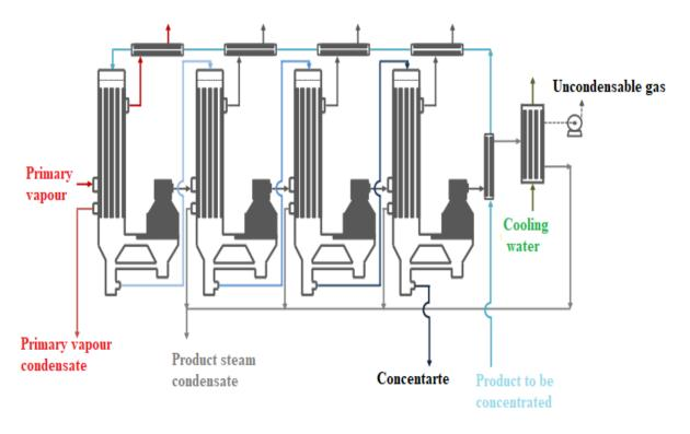
Figure 2.1: Multiple effect evaporator.[1]
