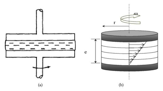
Figure 3.5: Parallel-plates rheometer [8].
