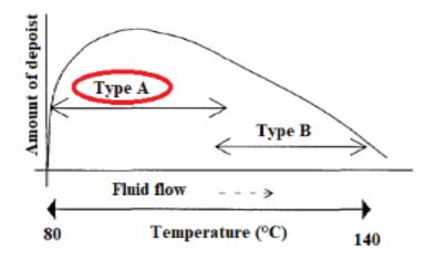
Figure 2.3: Distribution of A and B fouling deposit type with temperature along flow path .[3]
