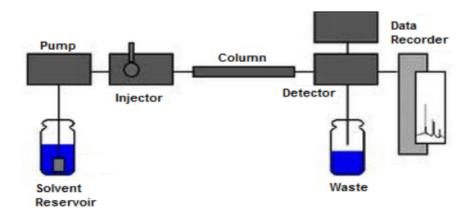
Figure 2.6: Operating principle of HPLC. [7]
