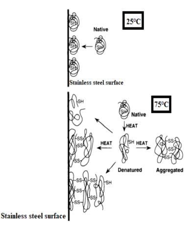
Figure 2.5: Adhesion mechanisms of  $\beta$ -Lg onto the stainless steel surface. [6]
