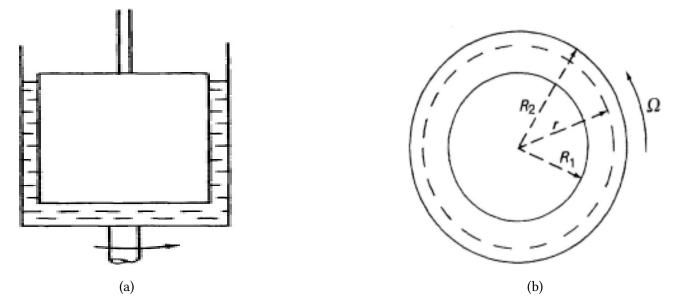
Figure 3.4: The concentric cylinder rheometer (side view on left and top view right) [8]
