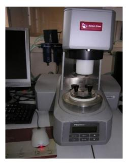
Figure 3.3: Rheometer (Physica MCR 301 series: Anton Paar GmbH).
