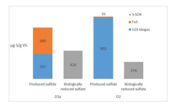
Fig 3: Comparison between sulfide production (either as  $H_2S$  in biogas or precipitated FeS) and biological sulfate reduction, for both first stage (D1a) and second-stage (D2) digestion. Values obtained from batch tests.
