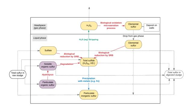
Fig.1: Sulfur species conversions during anaerobic digestion. Biological, chemical and physical reactions are indicated by red, green and blue colours. Organic and inorganic sulfur species are specified by yellow and purple colours. The dashed line shows the distribution of total sulfur in the raw sludge entering anaerobic digestion, and the composition of total sulfur in the digested sludge.
