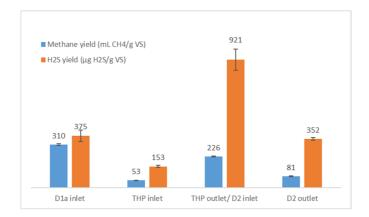
Fig 4: Profile of gaseous methane yield (mL CH<sub>4</sub>/g VS) and hydrogen sulfide yield ( $\mu$ g H<sub>2</sub>S/ g VS) in the different stages.
