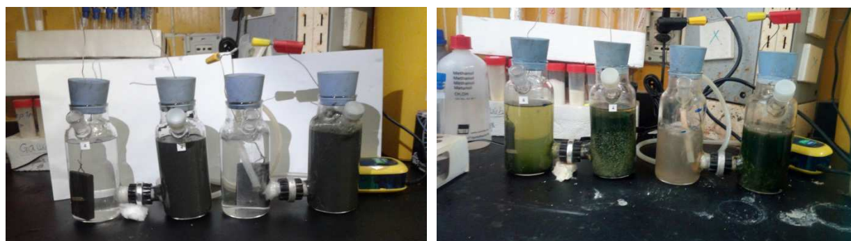
Figure 1 : sediment microbial fuel cell with anodic chamber fills with Mariout Lake sediment (sampling point 2) and cathodic chamber fill with water at the beginning (photo on the left) and after 45-day run (photo on the right). On the left of each photo the control cells (open circuit) and on the right the test cells (closed circuit).
