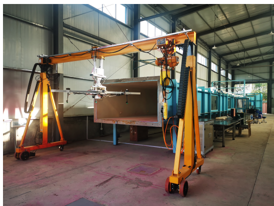
FIGURE 3 The UASS spraying test bench in South China Agricultural University.
