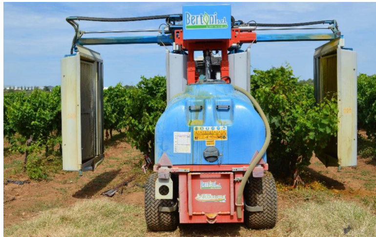
FIGURE 1. Air assisted tunnel sprayer (Acrobaleno, Bertoni®) fitted with air injection flat fan nozzles.
