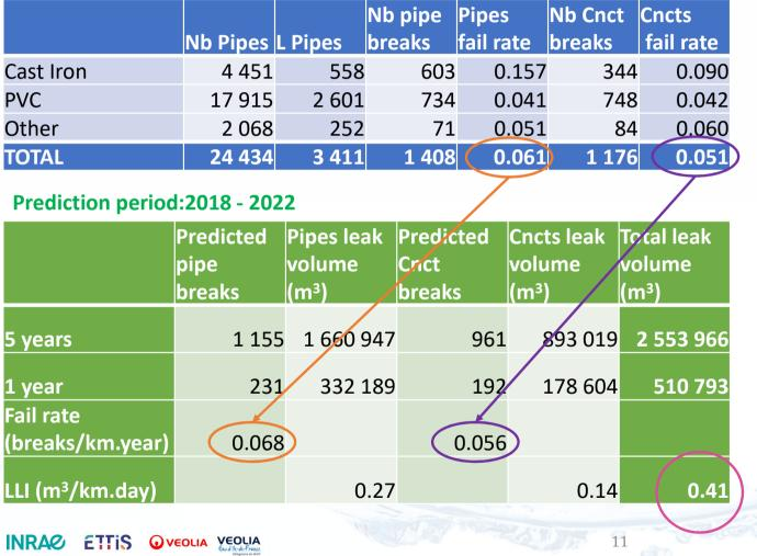
Break rates on pipes and connections are rising
