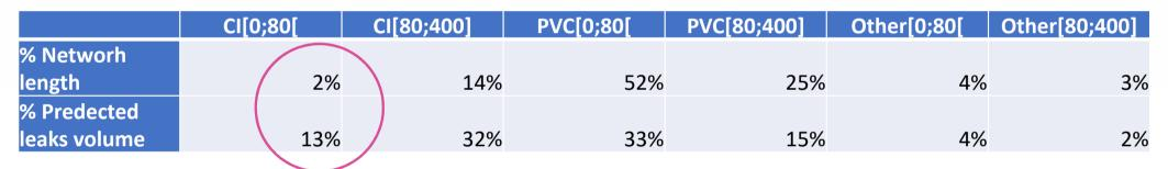
• Small diameter cast iron pipes represent 2% of the network length but are responsible for 13% of the volumes lost by detectable leaks.
