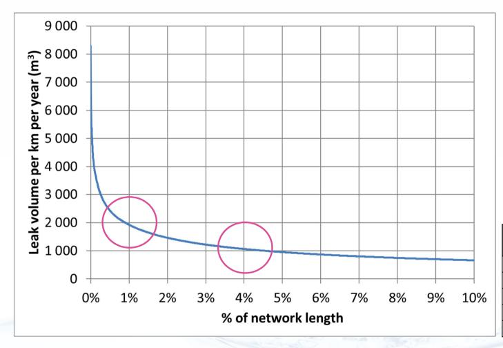
Pipe sections being sorted by decreasing risk of leakage, the volume of detectable leakage avoided per km of network renewed decreases rapidly:
