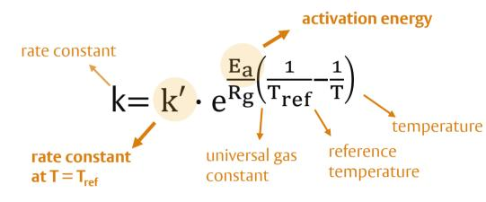
How to develop a kinetic model:
