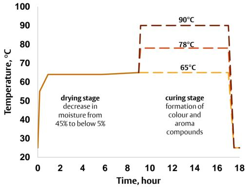
The drying stage was kept constant for all experiments. Isothermal curing stage in order to understand the effect of Multi-response kinetic modelling
