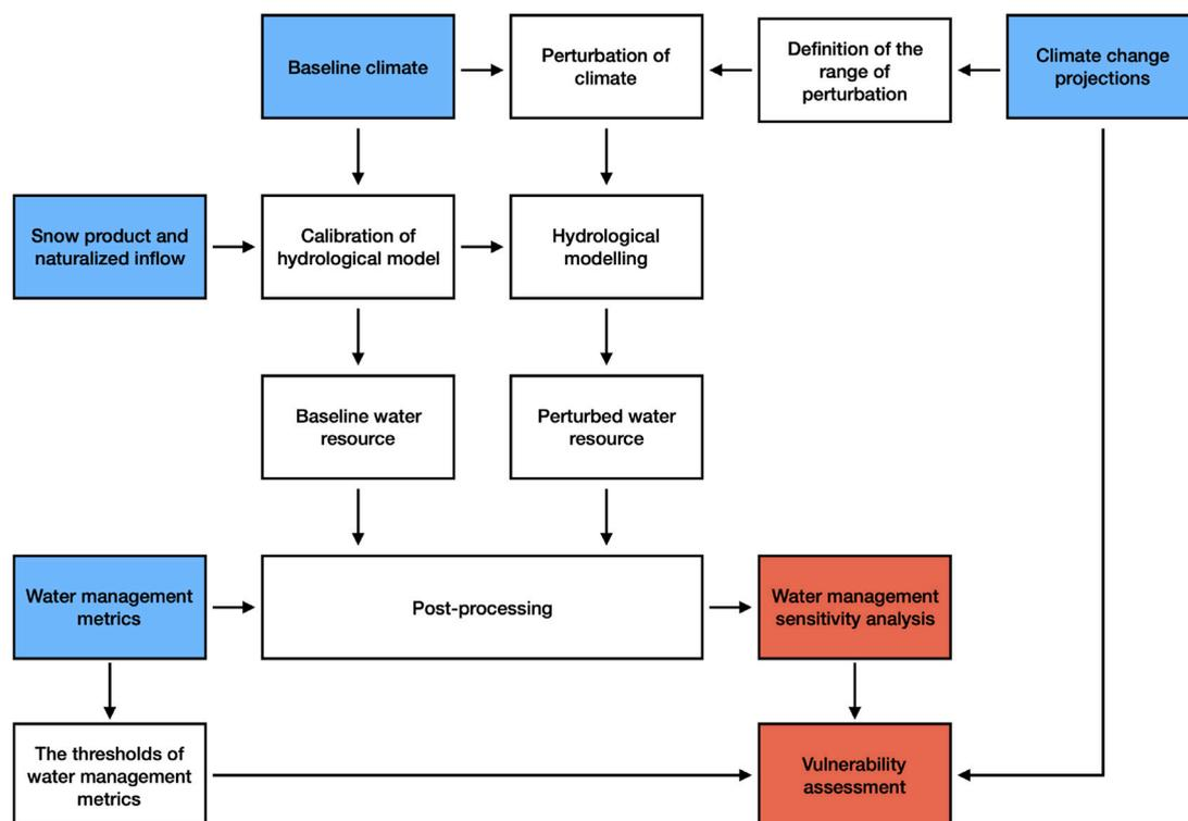
Fig. 2. The Scenario Neutral framework is applied to assessing the vulnerability of water management in the study area. The inputs and outputs are labelled in blue and red, respectively.
