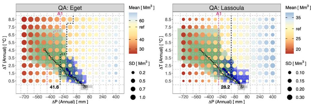
Fig. 9. The adaptation strategy of increasing the current turbine efficiency by 10% (A1) for the Eget and Lassoula systems.
