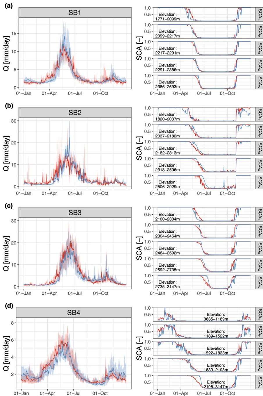
Fig. 4. Observed (red) and simulated (blue) median Q (left) and SCA (right) regimes for SB1(a), SB2(b), SB3(c), and SB4(d). The ribbon area in Q regime represents the percentile range of 25% and 75%. The SCA regimes are displayed for the five elevation bands. The observed/simulated period for SB1, SB3, and SB4 is from 01/2001 to 08/2014 while the observed/simulated period for SB2 is from 07/2014 to 07/2018.
