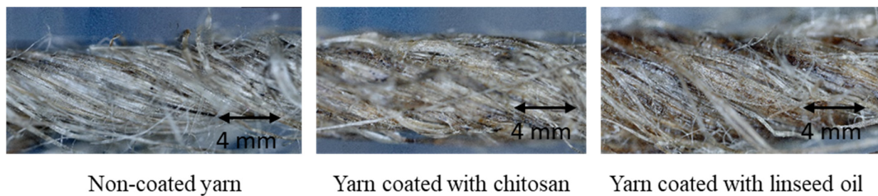
Figure 5. Microscopic representation of a non-coated yarn and yarns coated with chitosan or linseed oil.
