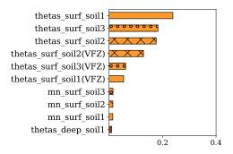
**Figure 8:** Aggregated sensitivity indices (ASI). Ten input parameters with the highest ASI are reported. The color and filling of the bars represents the nature of the input parameters as in Figures 1, 6 and 7.
