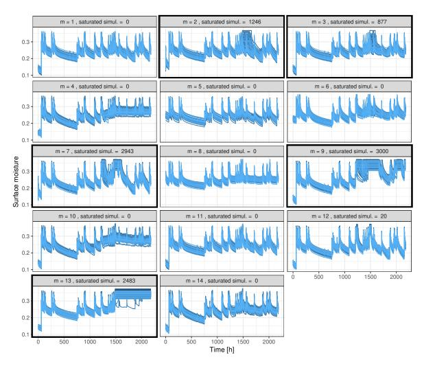
Figure 9: The first 100 output time series for all plots m=1..14 (out of 3000 simulations). The number of simulations presenting a saturated soil surface for longer than 100 hours are denoted next to the plot number (previously seen in Table 1). The plots considered belonging to the group  $\mathcal{G}_{sat}$  have a bold black frame.
