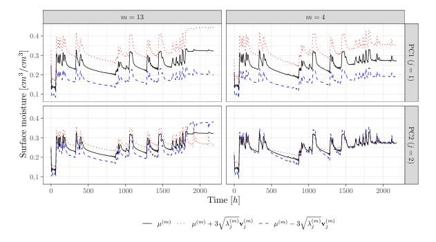
Figure 3: Perturbations on the first two PCs of plots  $m=4 \notin \mathcal{G}_{sat}$  on the left column and  $m=13 \in \mathcal{G}_{sat}$  on the right column. The top row shows the perturbations in the direction of PC1, the bottom row shows the perturbations on PC2. The mean of the sample outputs is presented with a solid black line. The red dotted line and the blue dashed line represent the output that is three standard deviations away from the mean in the direction of the corresponding PC.
