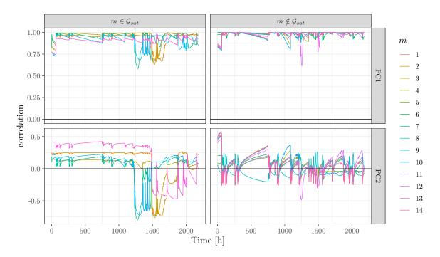
Figure 4: Correlations between the principal component scores  $H_j^{(m)}$  and the output soil moisture at time t, for each PC (rows), and for each plot m (curve color). The first column reports the plots  $m \in \mathcal{G}_{sat}$  and the second column  $m \notin \mathcal{G}_{sat}$ .
