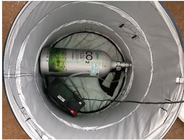
Figure 6. Inside view of a BG-Sentinel trap containing a battery and a CO 2 bottle.
