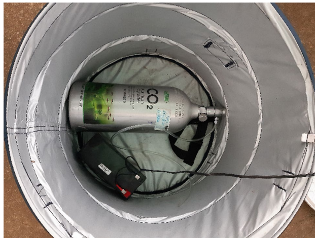
Figure 6. Inside view of a BG-Sentinel trap containing a battery and a CO 2 bottle.
