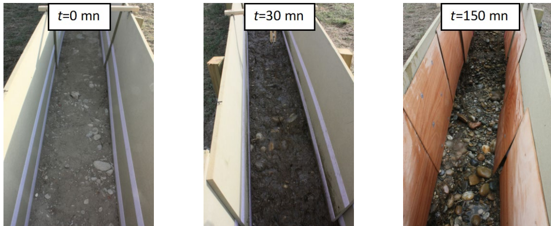
Figure 12. Erosion sandy gravel, between t = 0 and t = 150 min (channel 1).
