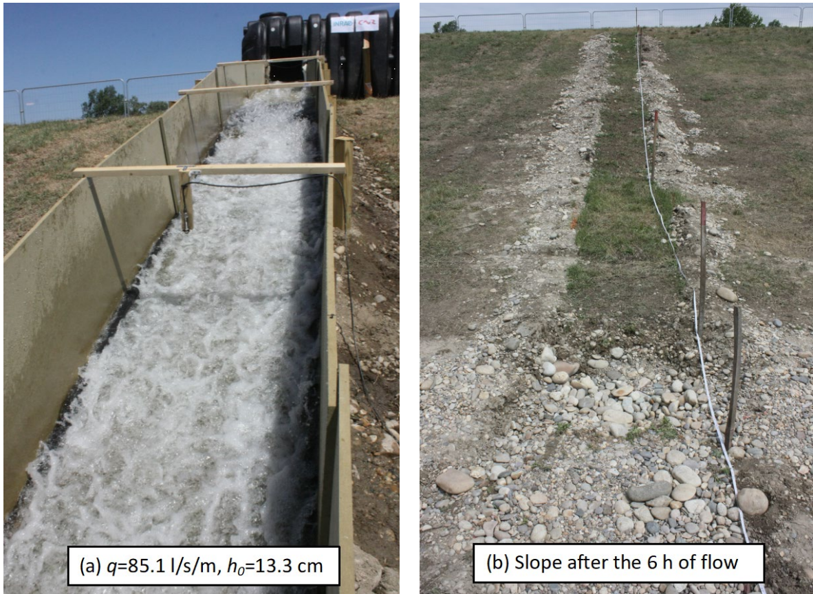
Figure 6. (a) Flow corresponding to q=85.1 l/s/m and h_0 = 13.3 cm. (b) Slope after the 6 h of flow.
