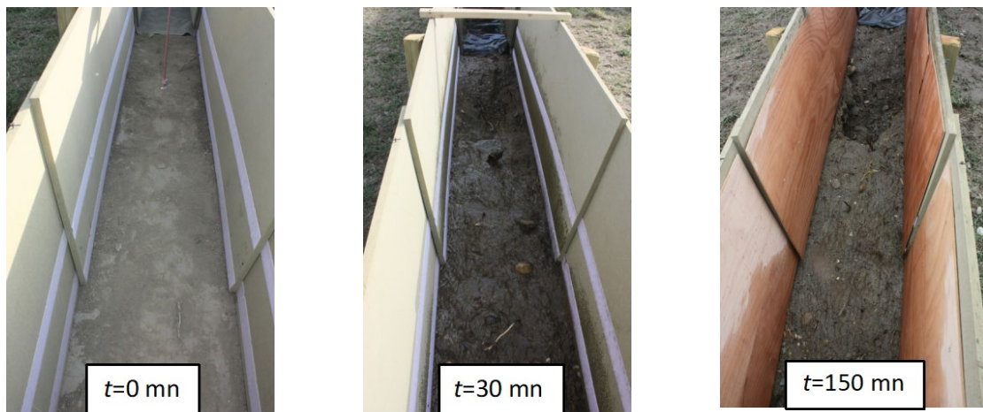
Figure 11. Erosion of compacted sandy silt, between t = 0 and t = 150 min (channel 1).
