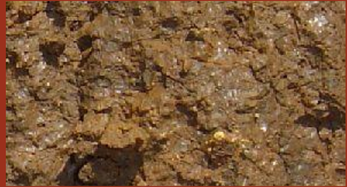
Large aggregates with bio-porosity = water could easily run between them
