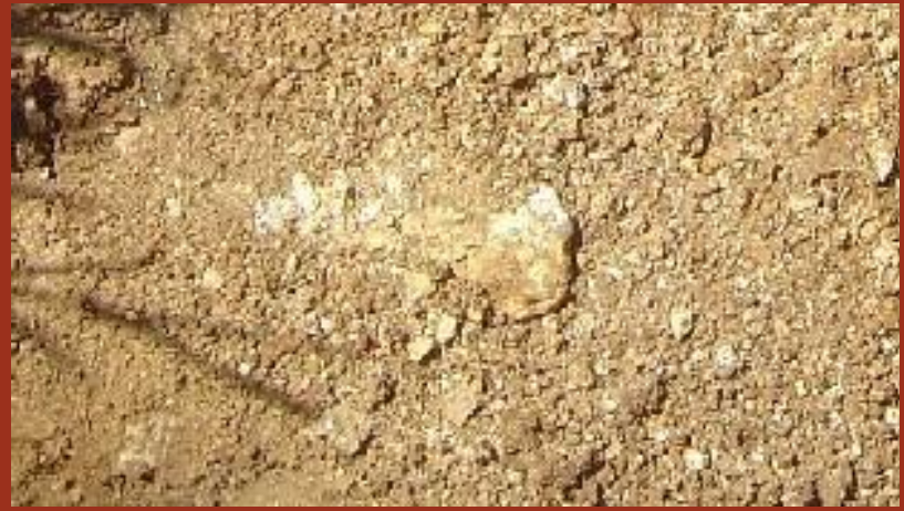
Weathered limestone : high hydraulic conductivity due to important fracturation and weathering processes
