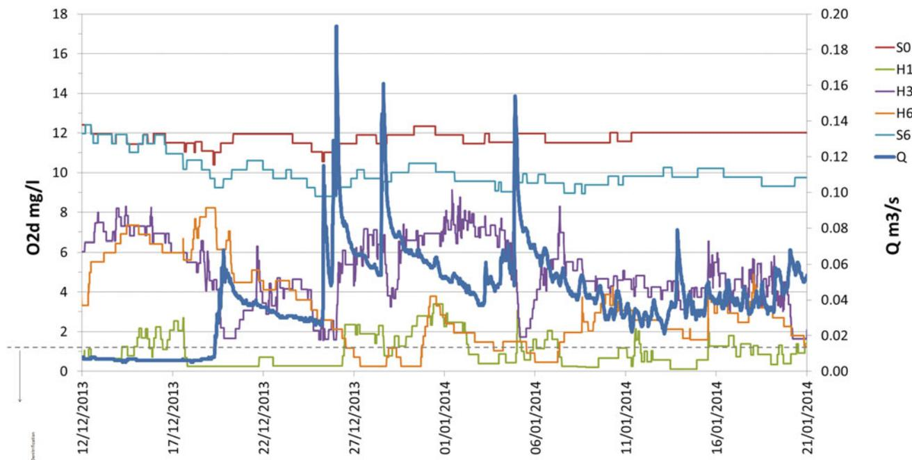
**Fig. 2** Variations of the dissolved oxygen concentration with time and space at wells H<sub>1</sub> to H<sub>6</sub> in the constructed riffle 1. ES00 stands for surface dissolved oxygen concentration. The dash line of 1 mg/L is the threshold for the denitrification process
