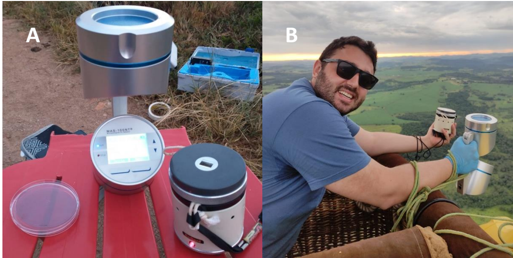
566 Supplementary Figure 1 – Fungal PBAPs sampling using the Microbial Air Monitoring 567 System (MAS100) and the portable Burkard air sampler at (A) ground level and (B) 300 m in 568 the hot-air balloon above the region of Arceburgo city, Minas Gerais state, Southeast Brazil, 569 during the fieldwork campaign between the 08 th to the 11 th of March 2022. Photos: MC 570 Mantoani and LCC Guerra.
