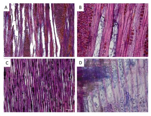
**Fig. 3** Wide field light microscopy observations. Representative examples of trypan blue staining of fungal hyphae in tangential sections of Beech wood (**a**, **b**) and in radial sections of Scot Pine (**c**, **d**). Images were acquired using  $10 \times /0.25$  NA (**a**, **c**) or  $40 \times /0.65$  NA (**b**, **d**) Plan C N objectives (Olympus).
