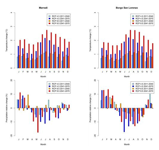
**Figure 3.** Absolute change (°C) in monthly mean air temperature (top graphs) and relative change (%) of monthly cumulated rainfall (bottom graphs) generated in the two study sites with the RCM ensemble (14 models) for two climate scenarios (RCP4.5, RCP8.5) and two periods–2011–2040 (ongoing) and 2041–2070 (mid-future)—over the baseline period 1981–2010 (near past).
