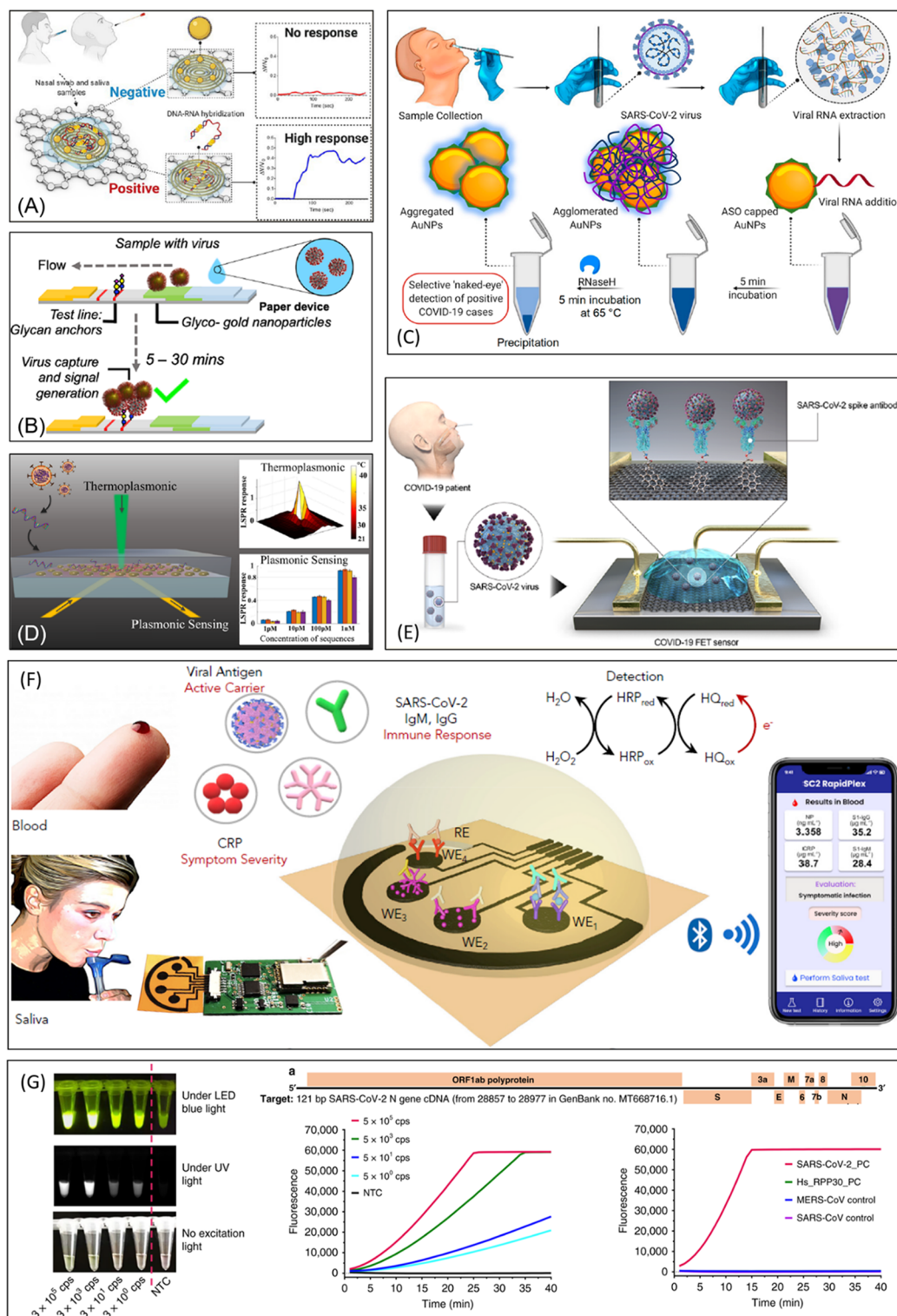
Figure 2. Examples of nano-biosensors for the detection of the SARS-CoV-2 virus and published in 2020. (A) Electrochemical paper-based interdigitated device for N gene detection using graphene and AuNPs. 52 Adapted with permission from ref 52. Copyright © 2020 American Chemical Society. (B) Spike protein lateral flow device using AuNPs and glycan anchors. 53 Adapted with permission from ref 53. Copyright © 2020 American Chemical Society. (C) Colorimetric (plasmonic) viral RNA detection method with the use of DNA-functionalized AuNPs. 56 Adapted with permission from ref 56. Copyright © 2020 American Chemical Society. (D) Thermoplasmonic device for the detection of membrane, spike, and nucleocapsid protein genes with DNA immobilized on 2D nanoislands. 57 Adapted with permission from ref 57. Copyright © 2020 American Chemical Society. (E) Graphene-based FET for real-time immune-based spike protein detection. 58 Adapted with permission from ref 58. Copyright © 2020 American Chemical Society. (F) Multiplexed electrochemical detection on laser-engraved graphene electrodes. 60 Adapted with permission from ref 60. Copyright © 2020 Elsevier. (G) CRISPR-based ultrasensitive fluorescent detection of two sites of the viral RNA genome. 64 Adapted with permission under a Creative Commons Attribution 4.0 International License from ref 64. Copyright © 2020 Springer Nature.
