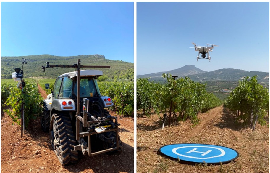
Fig. 2 Pictures of vineyard-based data collection with different sensors during the survey. Left: two vehicle-mounted sensors, SpectroSense + GPS and CropCircle, for measuring canopy reflectance; and Right: The Phantom 4 Pro UAV in use within the vineyard to collect proximal imagery. An on-site weather station is also shown in the left image
