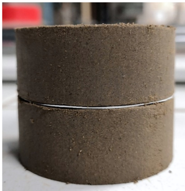
Fig. 4. Matric suction measurement by contact filter paper method.
