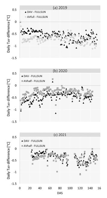
**Fig. 4.** Differences in the daily means of air temperature ( $T_{air}$ ) between AV and FULLSUN plots for 2019 (a), 2020 (b) and 2021 (c). In 2019 the two monitored AV plots were DAV (west) and AVfull, while in 2020 and 2021 the two monitored AV plots were DAV (west) and AVhalf).
