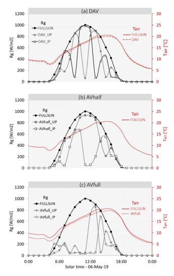
**Fig. 5.** Hourly dynamics of the incident global radiation (Rg) and air temperature for the DAV (a), AVhalf (b) and AVfull (c) devices, in comparison with FULLSUN conditions, showing differences between the IP (inter panel) and UP (Under-Panel) positions, for the sunny spring day of May 6th, 2019 (Tair was not measured in AVhalf for 2019). For legibility, the curves corresponding to air temperature data are in red, and the curves corresponding to radiation data are in black.
