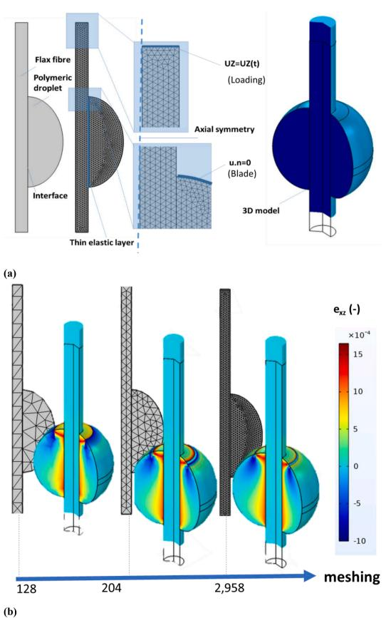
Fig. 4. (a) Illustration of the geometry and meshing used in the finite element computation, (b) mesh study showing the effect of the element size on the shear strain  $e_{xz}$ .
