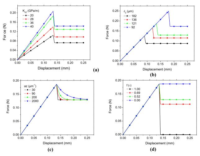
Fig. 6. Sensitivity analysis of the interfacial debonding law in PLA/flax system. Effect of (a) interfacial stiffness, (b) fibre–matrix complete separation displacement, (c) debonding propagation rate, (d) non-linearity factor.
