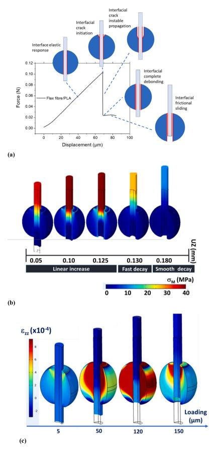
Fig. 5. (a) Schematic of the pull-out load–displacement curve with key stages describing the interface behaviour, Typical (b) von Mises stress ( $\sigma_M$ ), and (c) normal ( $\epsilon_{zz}$ ) strain components showing the main deformation stages of microdroplet test for flax fibre / MAPP composite.
