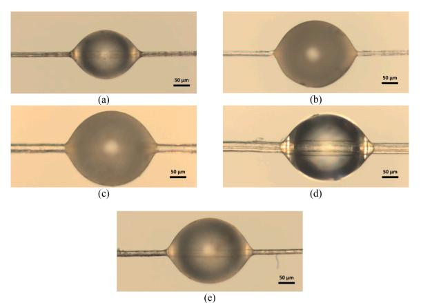
Fig. 2. Flax/ polymer microdroplet systems for the microdroplet test: (a) flax fibre/MAPP. (b) flax fibre /PBS, (c) flax fibre /PHA, (d) flax fibre/PLA, (e) flax fibre/PP.
