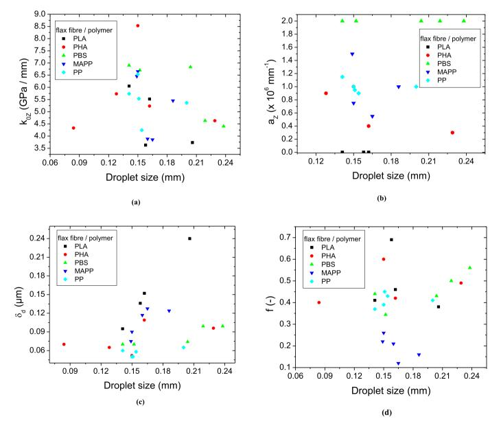
**Fig. 9.** Effect of droplet size on the interface parameters for all studied flax/polymer systems: (a) interfacial stiffness K0z, (b) debonding propagation rate az, (c) maximum fibre-matrix separation displacement  $\delta_d$ , (d) non-linearity factor f.
