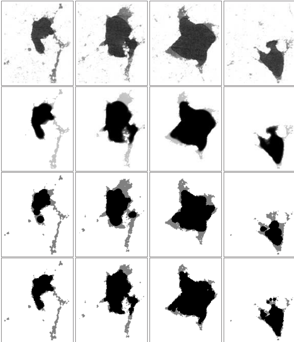
Figure 7: Comparison between SR- \mu CT (first row), LBM (second row) and MOSAIC (third and fourth rows) of the air-water distribution in the connected pore space of ROI p1bkk03a at different vertical sections z = 18, 24, 34 and 65 (from left to right). The water saturation index of the pore is 0.20 . Solid phase is in white, water is in light gray and air is in black. The third row corresponds to a threshold diameter value of 150 \mu\text{m} corresponding to h = -2 \text{ kPa} (resulting in S_w = 0.32 ) while the fourth row corresponds to a lower threshold value of 73.6 \mu\text{m} (resulting in S_w = 0.19 ).
