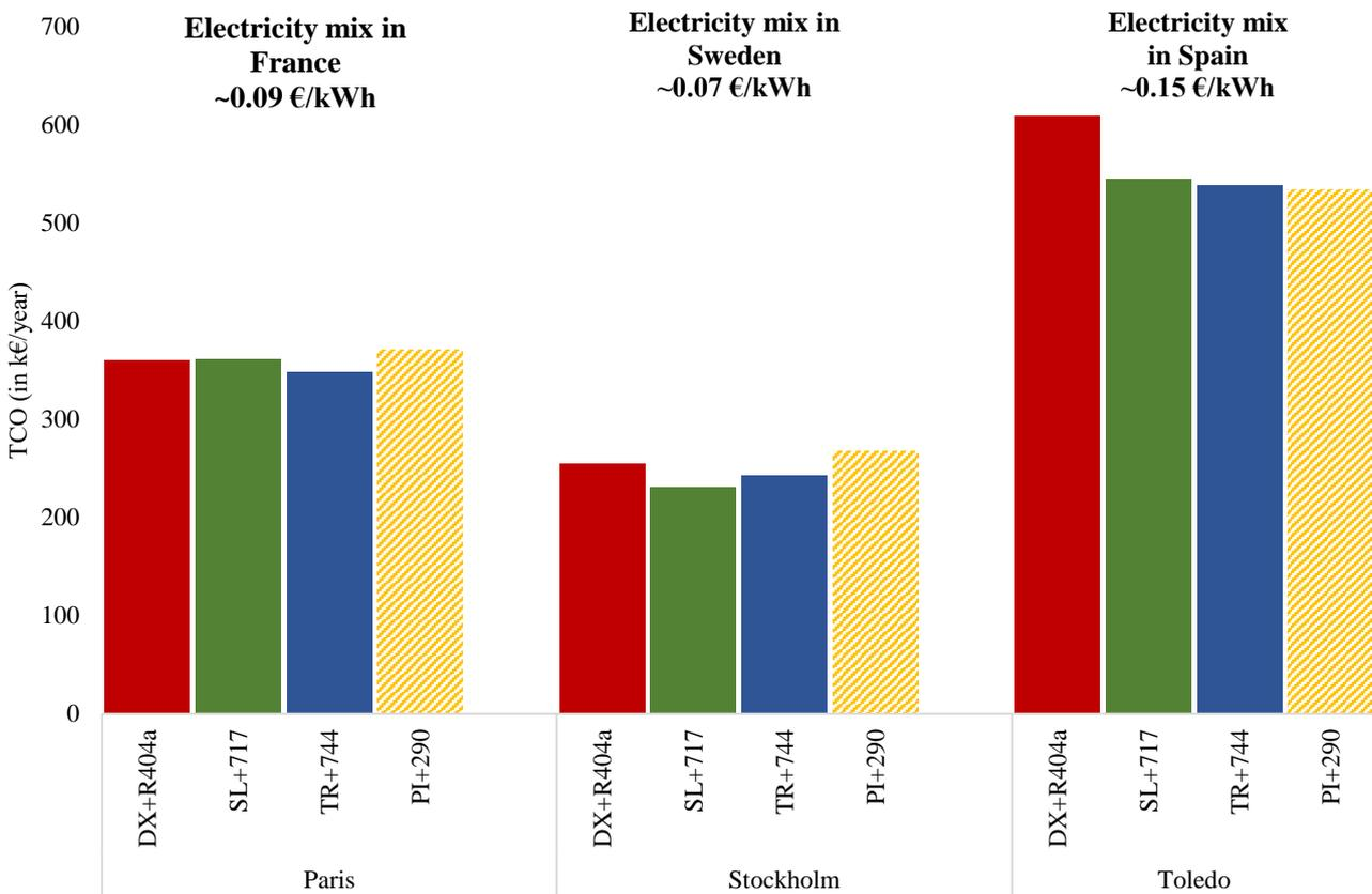
Figure 9. Average annual TCO calculated over ten years for a supermarket in three locations with four architectures: DX; SL; TR; PI (data of electricity mix from Eurostat).
