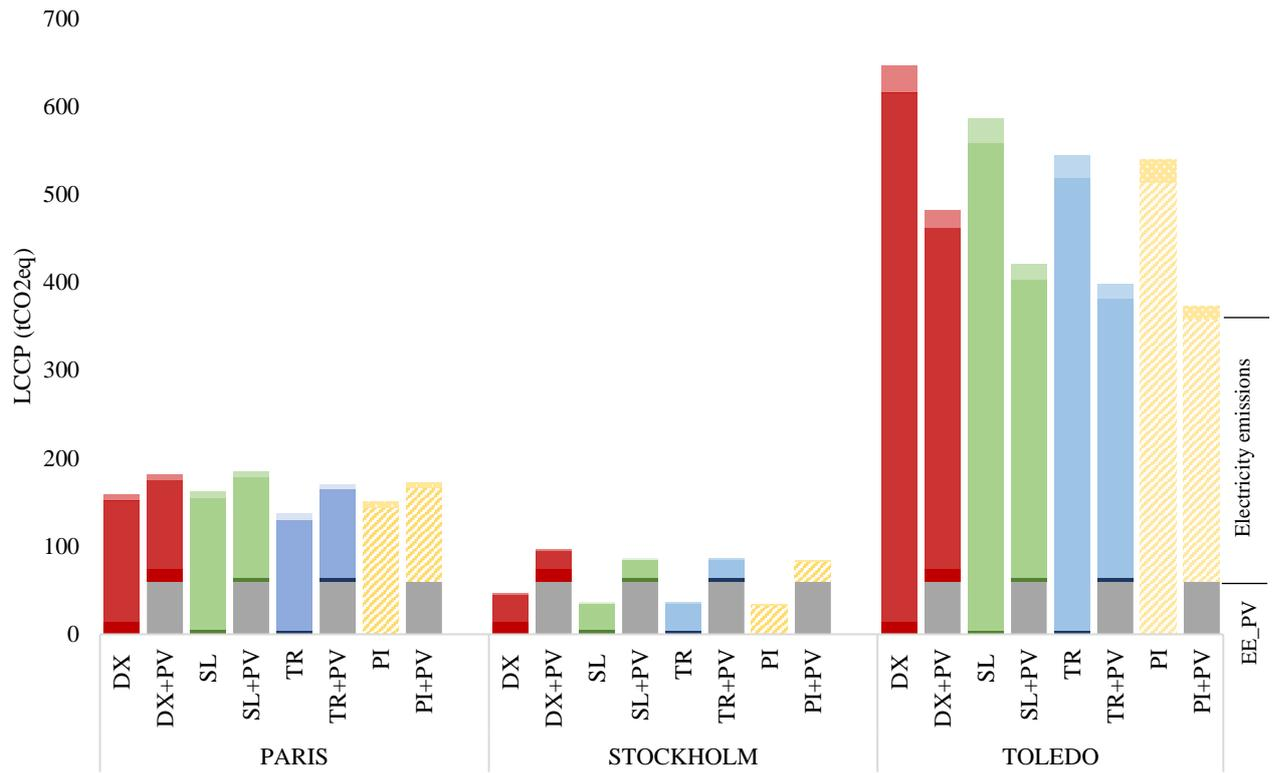
Figure 13. CO<sub>2</sub> emissions based on LCCP approach in the first year for the three locations and the four architectures (DX, SL, TR, PI) with and without PV (grey)
