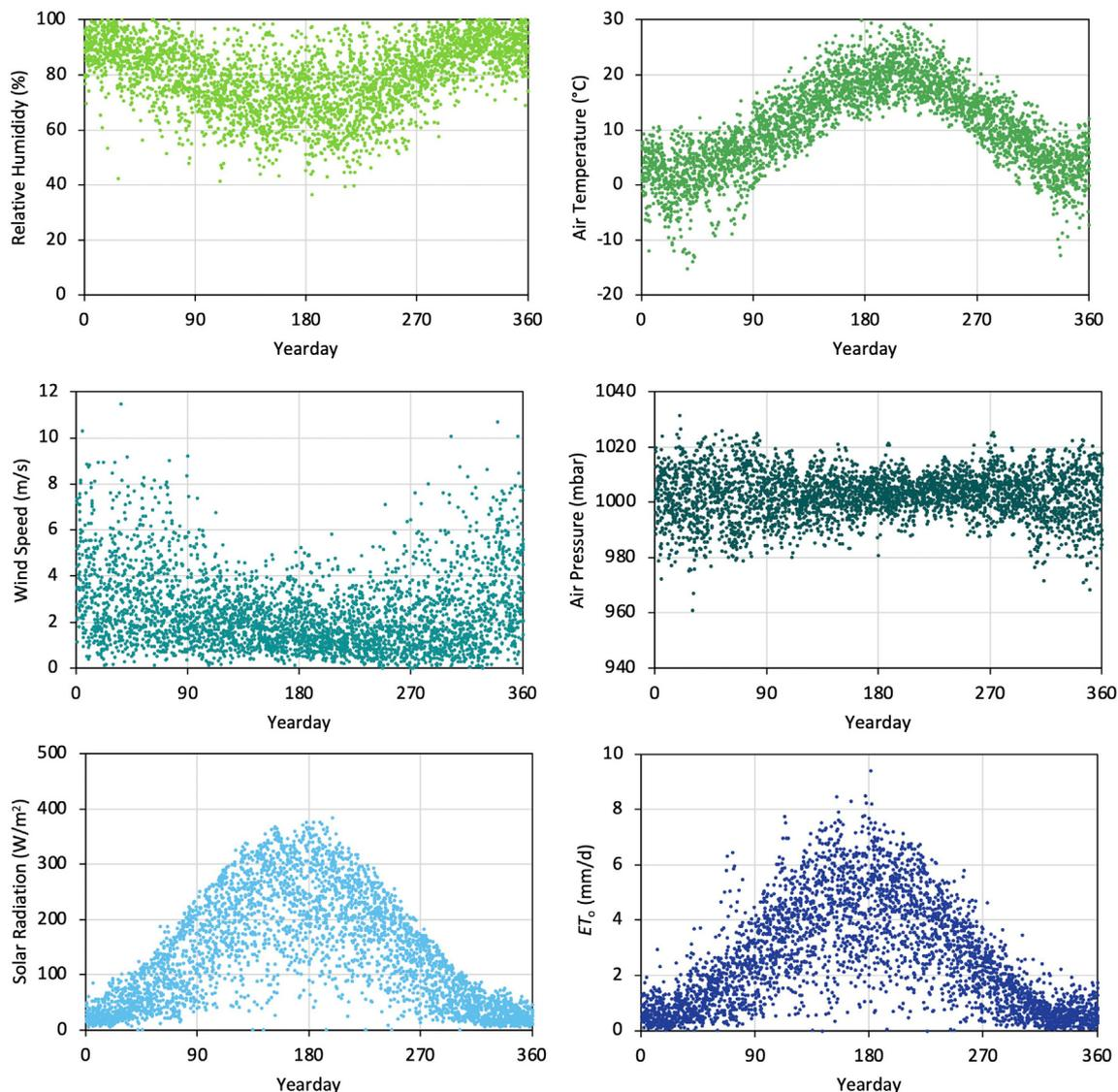
**Fig. 4.** Daily mean relative humidity, air temperature, wind speed, air pressure, solar radiation, and calculated Penman evapotranspiration ( $ET_o$ ) at the research platform in Langenreichenbach, Germany. Data shown are from August 2010–July 2020.
