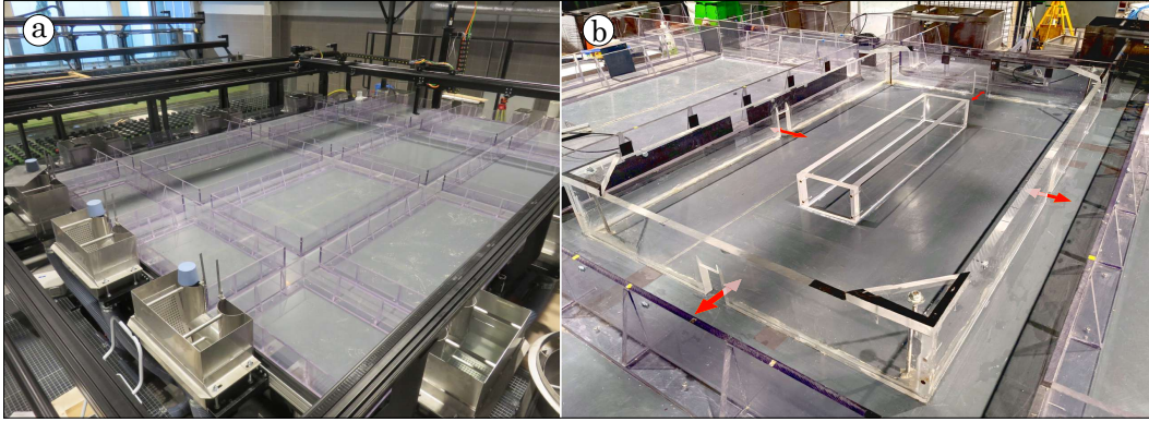
Figure 2: a) Overview of the Maquette Urbaine pour l'étude du Risque d'Inondation, MURI (Urban Model for the study of Flood Risk). b) Close-up of the city block with an opening in each of its sidewalls (conveyance porosity, \psi ), including a non-porous inner building that reduces the space available for storing floodwater volume (storage capacity, \phi ). The red arrows stand for flow exchanges between the streets and the city block through the openings.
