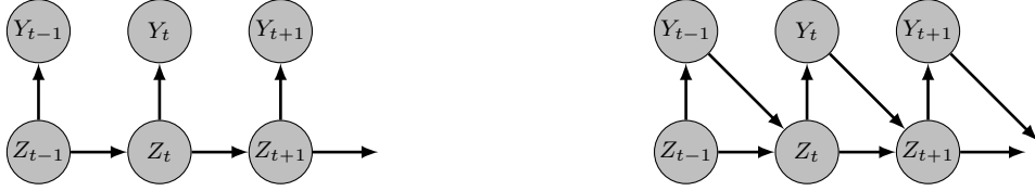
Figure 1. Graphical representation of conditional independencies in the chain (Z_t, Y_t) for an HMM (left) and for an OD-HMM (right).
