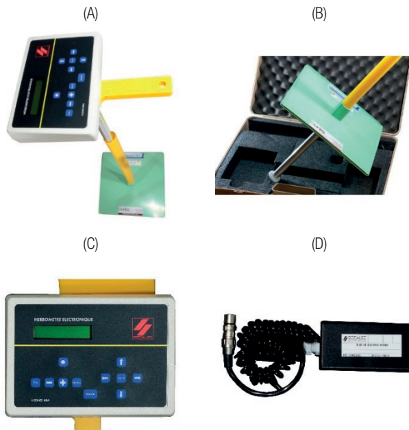
Figure 2: (A) HerboMETRE® and its elements. (B) Rising plate mounted on the yellow plastic tube around the aluminium axis tube. (C) Electronic ultrasound transducer. (D) Twelve volt battery. Photos: https://farm-store.eu/produit/herbo-metre/
