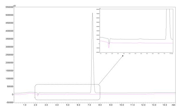
**Figure 1.** Reference chromatogram of pentobarbital sodium at a concentration of 150  $\mu$ g/mL (black curve) and blank sample chromatogram (pink curve).
