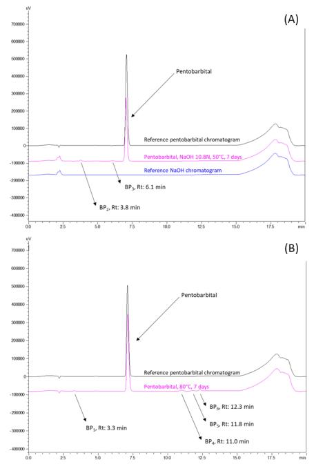
**Figure 2.** Chromatograms at 214 nm of breakdown products (BPs) obtained after forced degradations: (**A**) alkaline conditions of NaOH 10.8N for 7 days at 50  $^{\circ}$ C and (**B**) thermic conditions of 80  $^{\circ}$ C for 7 days. Rt: retention time.
