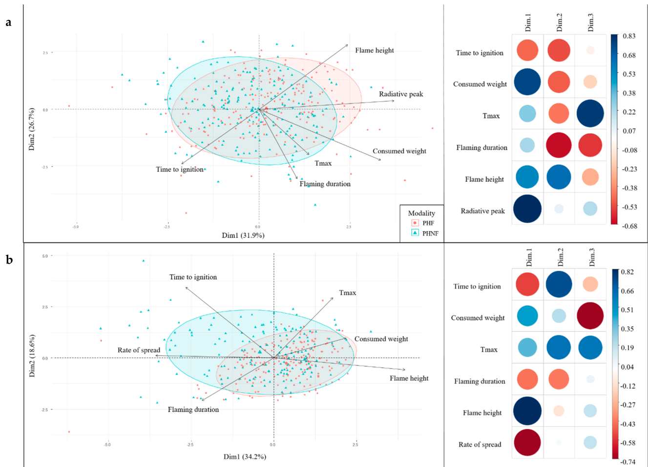
Figure 1. Biplots of principal component analyses (only the two first components (Dim) are shown) illustrating relationships between flammability variables (Tmax: maximum temperature) and fire modalities for P. halepensis ' shoot (a) and litter (b) flammability. Populations sampled in the high Fire recurrence modality (PHF) are circled in blue, and populations sampled in the No-Fire modality (PHNF) are circled in orange. The correlation plots indicate the regression coefficient of each trait on each component: the darker and larger the circle color and size, the stronger the correlation.
