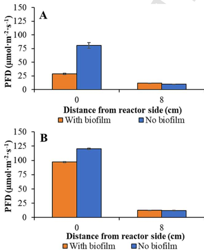
**Fig. 2.** Photon flux densities (PF<sub>D</sub>s) measured on the inner reactor wall and on the opposite side during Period II at days 57 (A) and 61 (B). The biofilm thickness (1–3 mm) was considered to be negligible for distance calculations.
