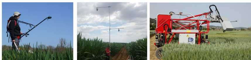
Fig. 3 Three acquisition systems used to build VegAnn. From left to right: handheld camera on the LITERAL device, camera equipped with a fish-eye lens and mounted on a probe, and cameras mounted on the Phenobile. The individuals consent to the publication of the images.
