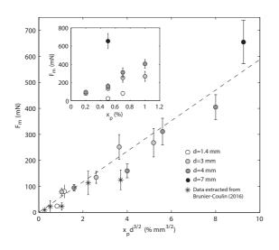
**Figure 2.** Micro-tensile force  $F_m$  as a function of  $x_p d^{3/2}$ . The dashed line stands for  $y = \alpha x$ , with the fit parameter  $\alpha = 59 \pm 7$ . Inset:  $F_m$  as a function of  $x_p$ .
