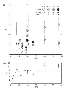
**Figure 6.** (a) Coordination number  $Z_c$  as a function of D/d. The caption indicates the meso-scale devices' size and the paraffin content. (b) Averaged values of  $Z_c$  as a function of D/d. The dotted line stands for the theoretical prediction from Eq.5.
