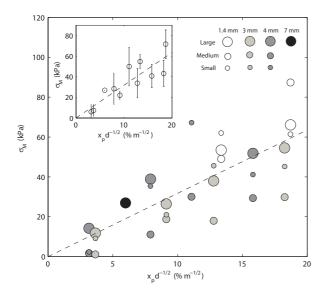
**Figure 5.** Macro-scale tensile stress  $\sigma_M$  as a function of the paraffin content  $x_p$  divided by  $\sqrt{d}$ . Inset: Averaged values. The dashed line stands for  $y = \beta x$ , with the fit parameter  $\beta = 3.2 \pm 0.4$ .
