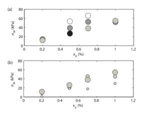
**Figure 4.** Macro-scale tensile stress  $\sigma_M$  as a function of the paraffin content  $x_p$ . (a) Large device with d=1.4 mm (white), d=3 mm (grey), d=4 mm (dark grey), and d=7 mm (black). (b) Large, medium and small devices (symbol size) with d=3 mm.
