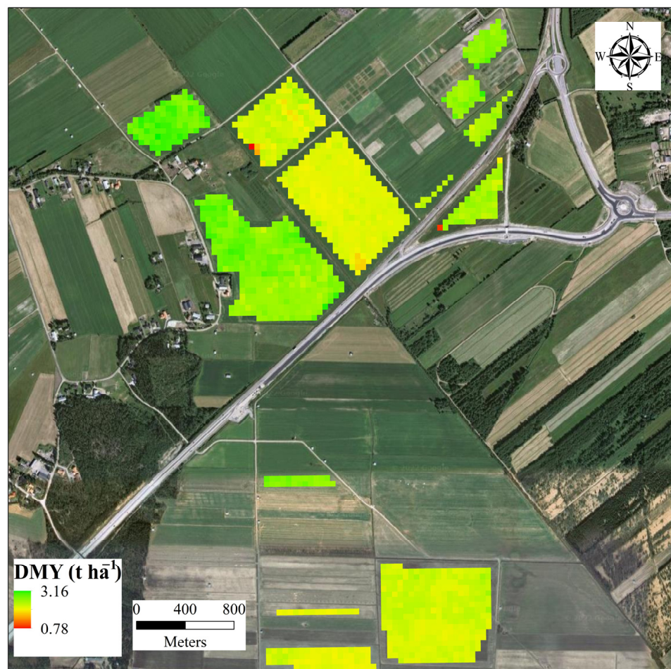
Figure 7. Layout of the estimated dry matter yield ( DMY ) for the first harvest from Sentinel-2 imagery obtained on 09 June 2019, one week before the first harvest using a selected RFR model, at Röbbäcksdalen field research station. The background imagery is obtained from Google Earth.
