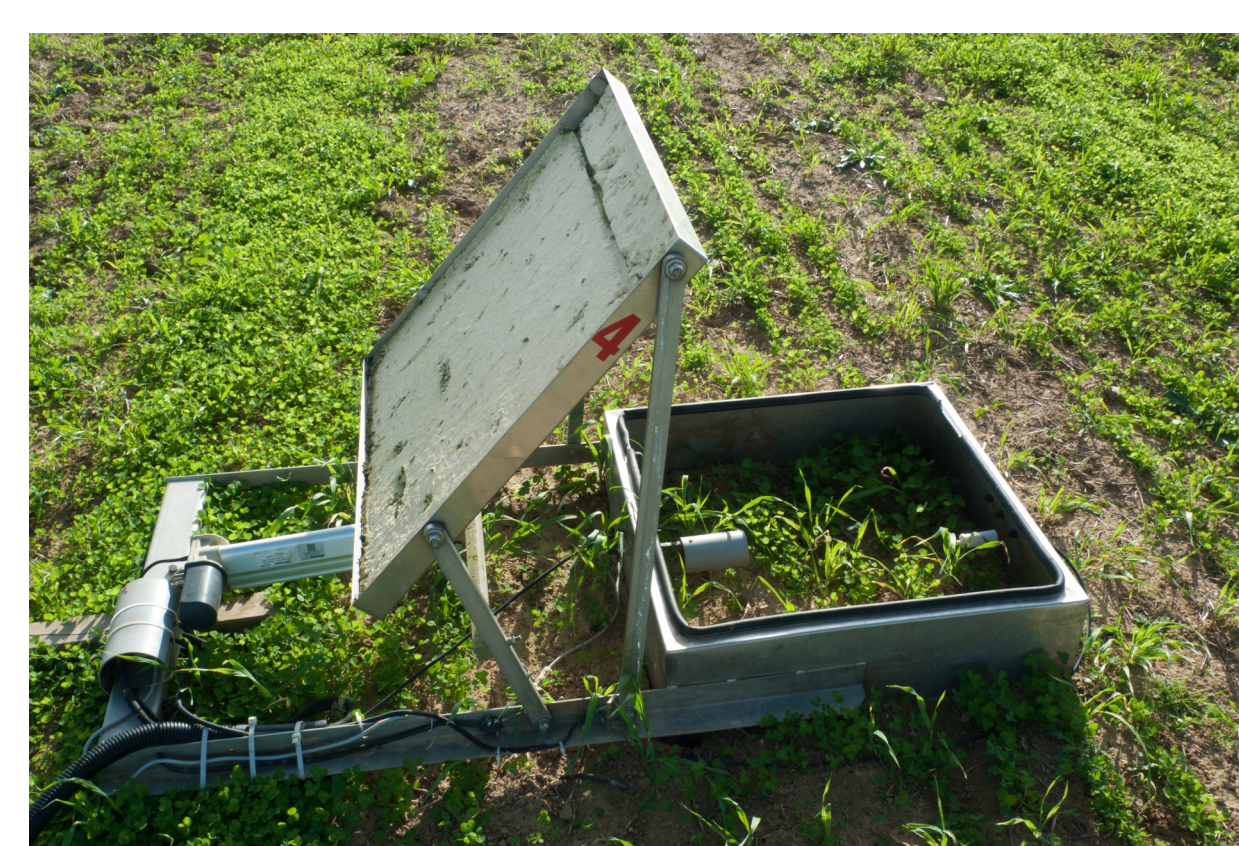
Fig. 2: the automatic chambers system measures N 2 O emissions
