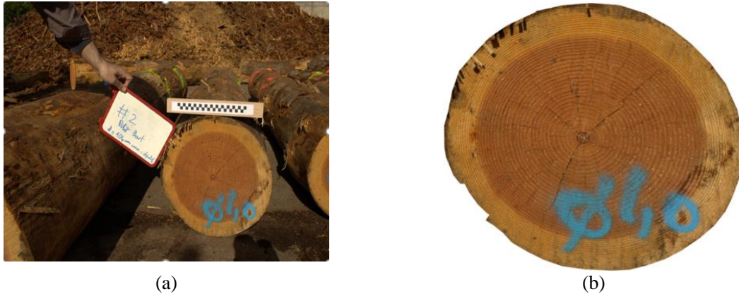
Fig. 1: Images of log #02: log end image taken on the log-yard ; the corresponding manually segmented log image.
