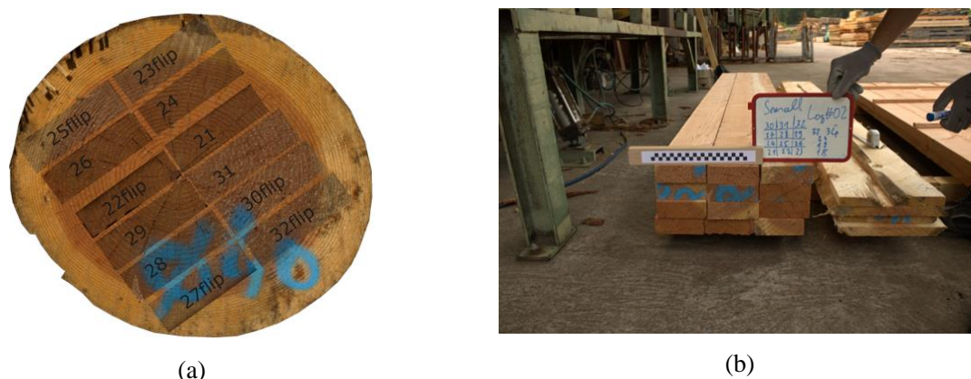
Fig. 2: (a) Manual positioning of the board end image for log #02 (flip means that the board end image had to be flipped to be in the right orientation); (b) A pile of boards from log #02.
