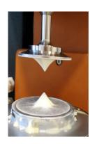
Probe-track test cohesion of high cohesive concentrates
