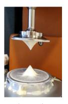
Probe-track test cohesion of high cohesive concentrates
