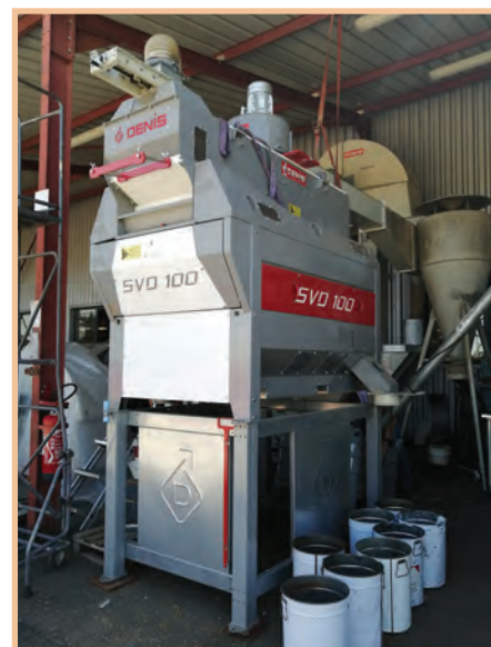
Figure 2 SVD100 vibrating cleaner from Etablissements Denis used to demonstrate the feasibility of the separation of species mixture and the resulting economic benefit (Picture from Patrick Bourrachot)
