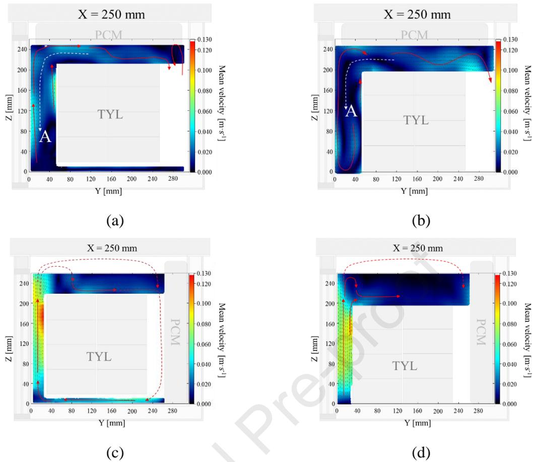
636 **Figure 4:** Measured air velocity field on the middle plane of a loaded box (a) PCM at the top,
