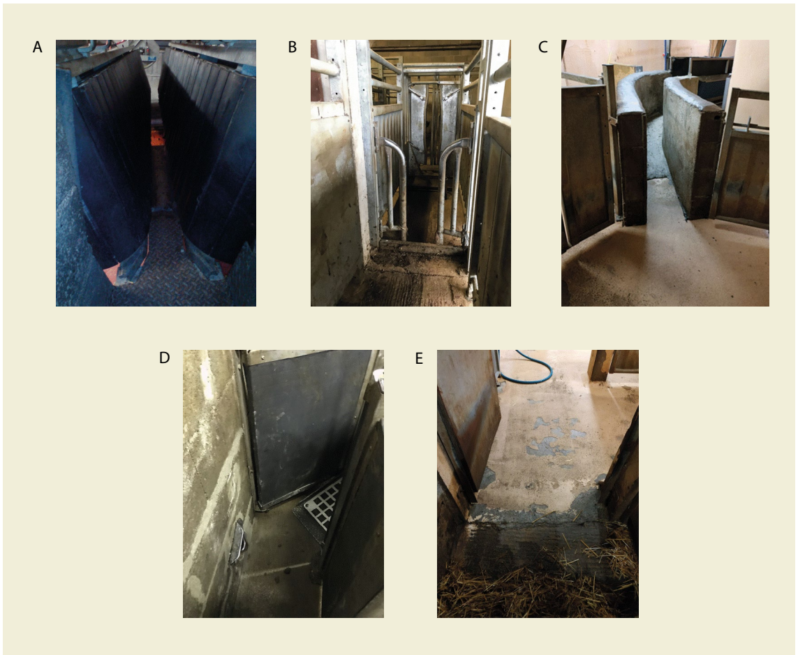
Figure 1.1. (A) Entrance of a pig restrainer. The negative points are that the area is too dark; the environment outside the restrainer is visible causing too many distractions for the animal; the false-floor is lacking in the restrainer, while it is known that the absence of a floor causes fear; and metal floors are inappropriate because they may vibrate and be noisy. (B) Cattle identification crush. The negative points are that the environment may be difficult to interpret for the animal because there are too many objects and shapes; the walls are too low allowing vision of the outside environment distracting the animals; there is insufficient light, with dark areas; the floor is non-homogeneous and there is a step at the entrance of the crush which may present obstacles for the animal; and the one-way backstop is little efficient. (C) Sheep entrance of a single file race towards the slaughter area. The negative points are that the reduction in the size of the entrance of the race is too abrupt; the environment outside of the race is too light, possibly distracting the animal; and the aspect of the floor changes which the animal may perceive as an obstacle. (D) Entrance of a pig restraining box. The negative points are that the corner is too sharp; the aspect of the floor changes which the animal may perceive as an obstacle; metal floors are inappropriate because they may vibrate and be noisy; and the concrete floor does not have a non-slip surface. (E) Sheep entrance to the slaughter area. The negative points are the complexity of the environment, which may be difficult to interpret for the animal; the presence of the water hose and the changing aspect of the floor, which may present obstacles for the animal. (Photo courtesy of C. Bourguet, Bureau ETRE, France)
