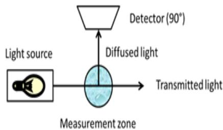
Fig. 1: Principle of meunier nephelometer used by Monod
