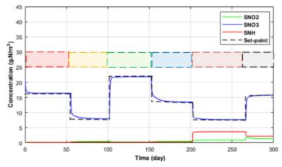
**Figure 3:** An open loop control strategy: switching each 50 days between the different configuration and input control values allows the control of the output concentrations of NH4 and NO3 in open loop (Aichouche, 2021).
