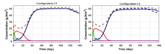
**Figure 5:** Closed-loop control of nitrogen needs for irrigation with C1 and C3 configurations - NO3 (blue), NH4 (green), NO2 (red) organic nitrogen (pink) concentrations, irrigation set-point (black dashed line) and total nitrogen in the effluent (brown dashed line).
