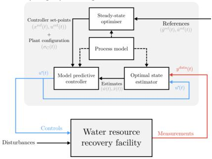
**Figure 6:** Output-MPC: Control architecture. The operation of the controller is based on the signals representing the state (x(t)), outputs (y(t)), disturbances (w(t)), and controls (u(t)) of the process. The function  $\sigma_C(t)$  represents the switching mechanism to select a plant configuration (C1-C6).
