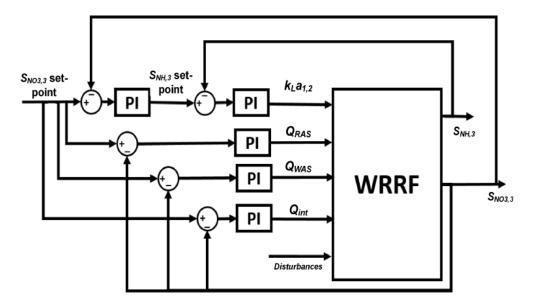
Figure 4b: Cascade control strategy #1 for the regulation of output nitrate concentration
