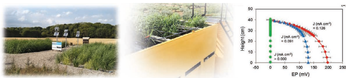
Fig. 1 Images of different full scale configurations for METland® technology in Spain and Denmark, and Electric Potential profile of electroconductive bed
