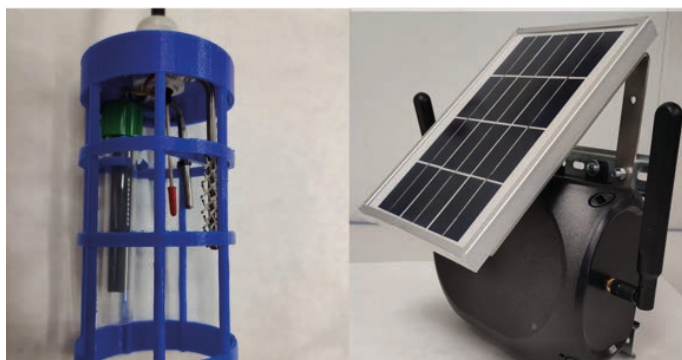
Fig. 1 A) IoT microbial electrochemical biosensor for in situ and online monitoring of water quality.
