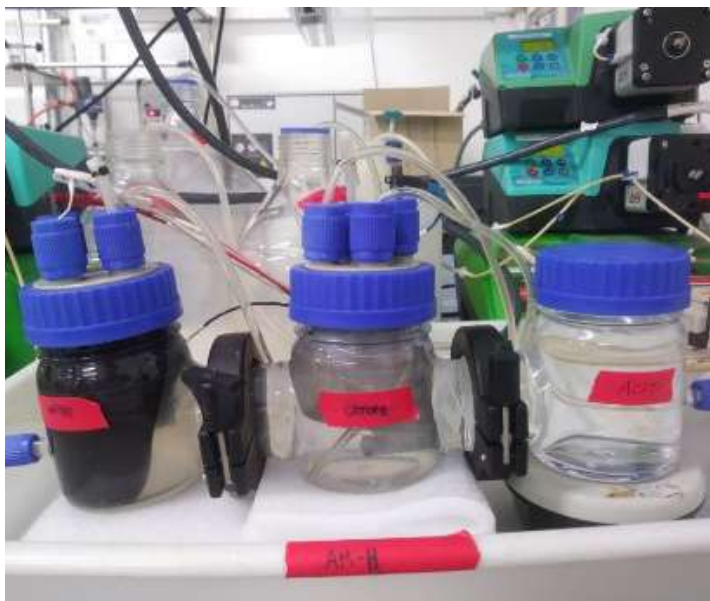
Fig. 1 Picture of the three compartment MEC. Anode, cathode and ammonia recovery chambers on the left, centre and right compartments, respectively.
